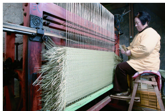
Fig17: Manufacturing process of Shichitoui tatami-omote(surface of tatami)
